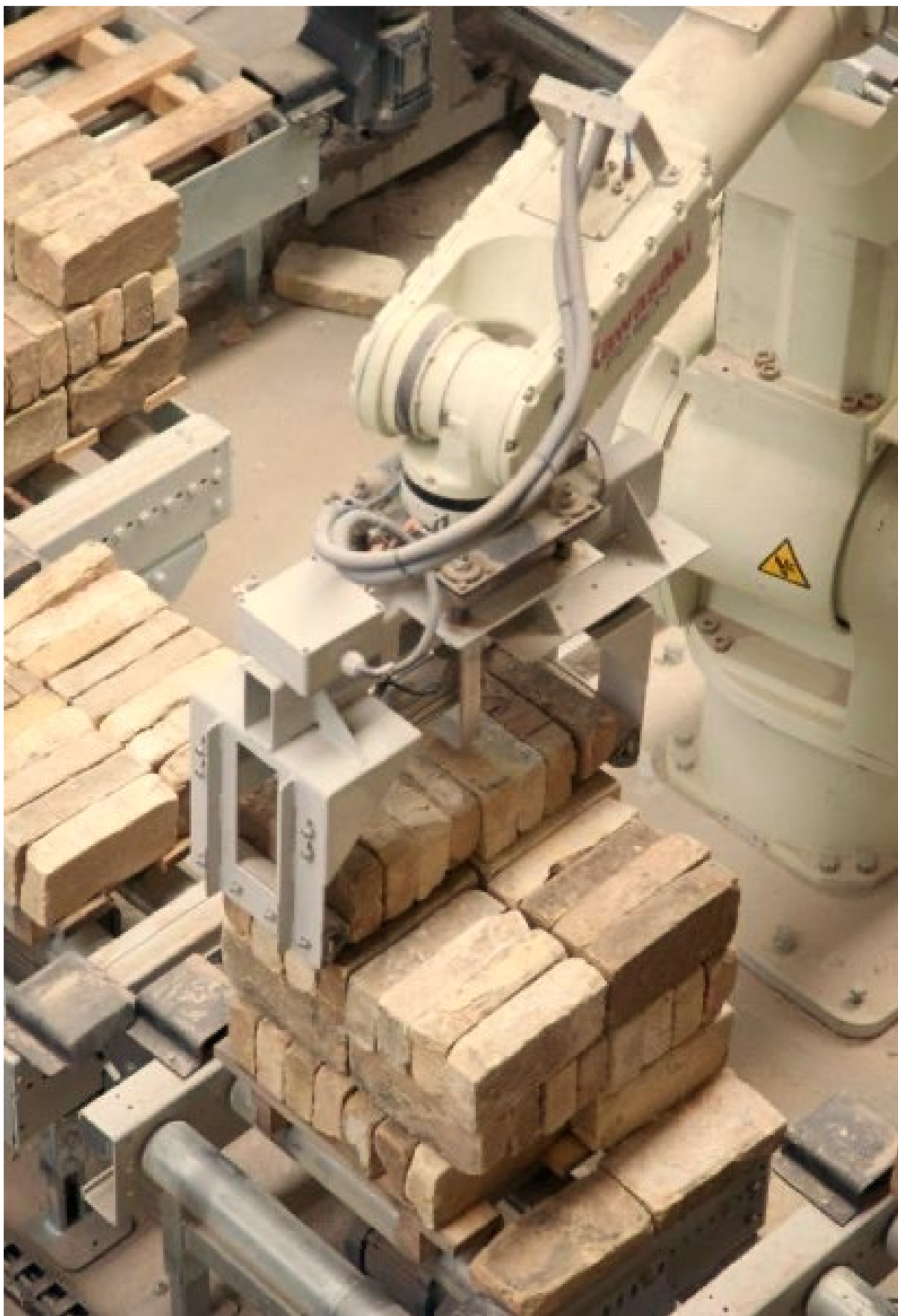
Robotized brick handling in Scandinavia (Web image 11)
