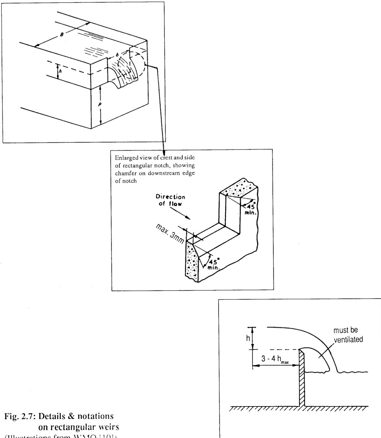
Fig. 2.7: Details & notations on rectangular weirs (Illustrations from WMO [10])
