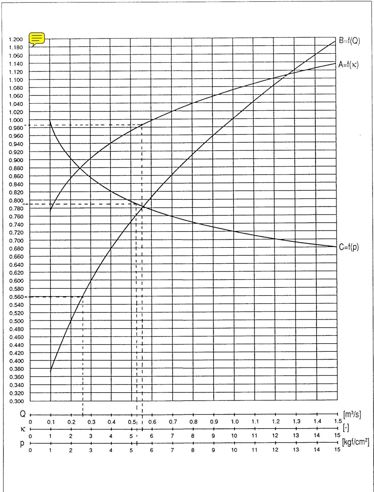
Fig. 2.14: Diagram for the pre-selection of the economically optimal penstock diameter
