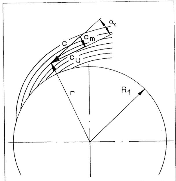
Fig. 1.11: Ideal flow conditions in the inlet
