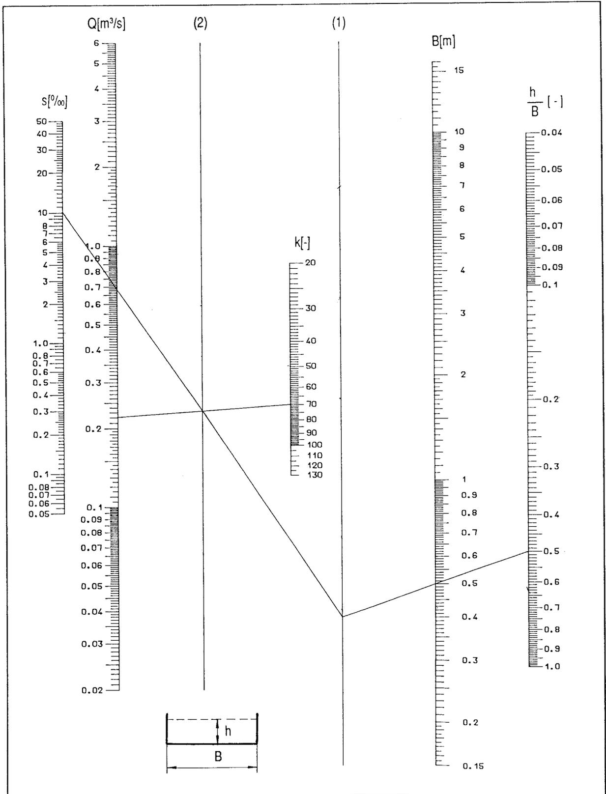
Fig. 2.3 : Flow in rectangular canal cross sections
