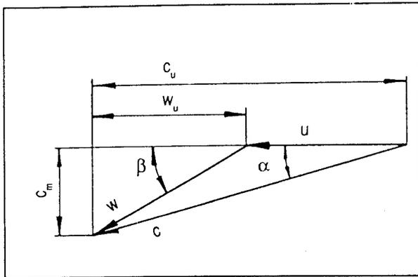
Fig. 1.5: Terms used in velocity triangles
