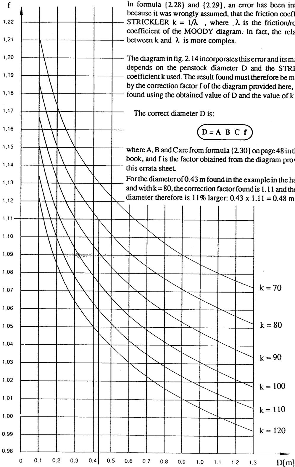
In formula (2.28) and (2.29), an error has been introduced because it was wrongly assumed, that the friction coefficient of STRICKLER  $k = 1/\lambda$ , where  $\lambda$  is the friction/roughness coefficient of the MOODY diagram. In fact, the relationship between  $k$  and  $\lambda$  is more complex.
