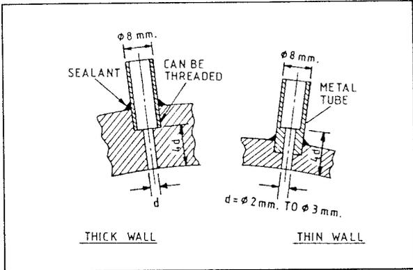
Fig. 3.9 : Single pressure tapping in PVC pipe
