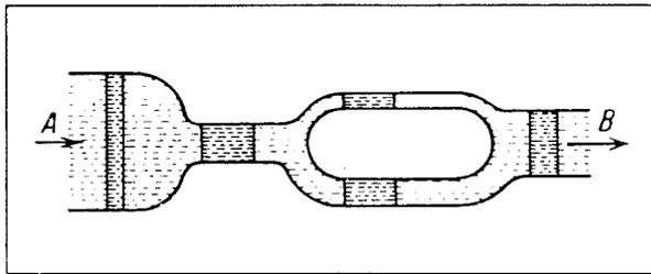
Fig. 1.1: Steady state flow
