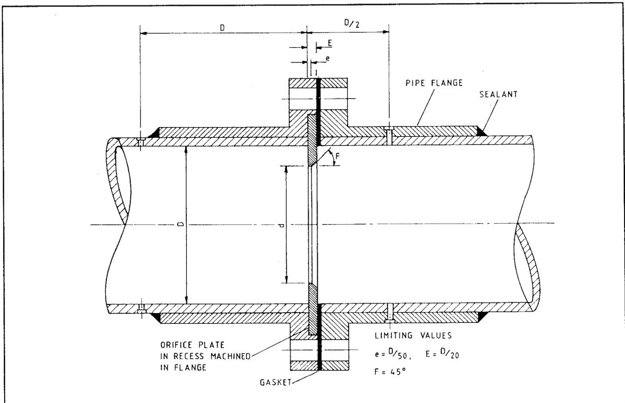
Fig 3.10 : Orifice meter in PVC pipe
