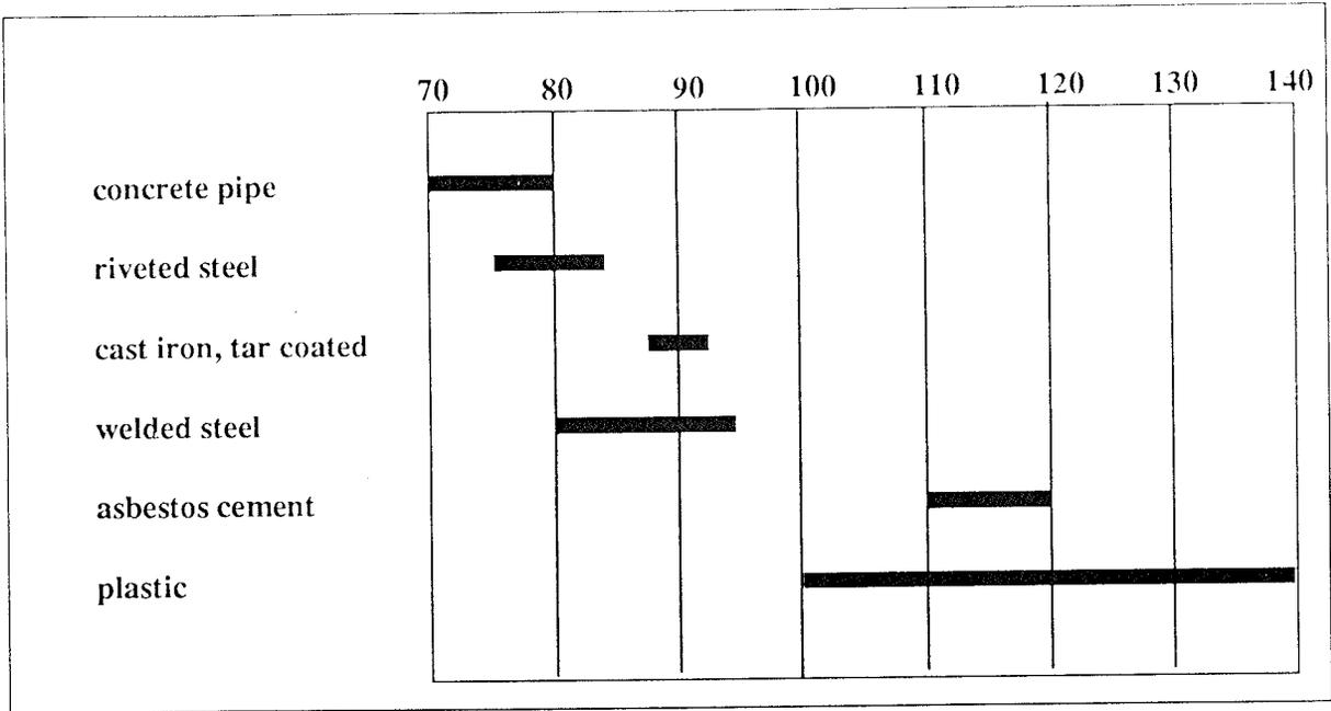
Fig. 2.10 : Friction coefficients k for penstock materials according to STRICKLER
