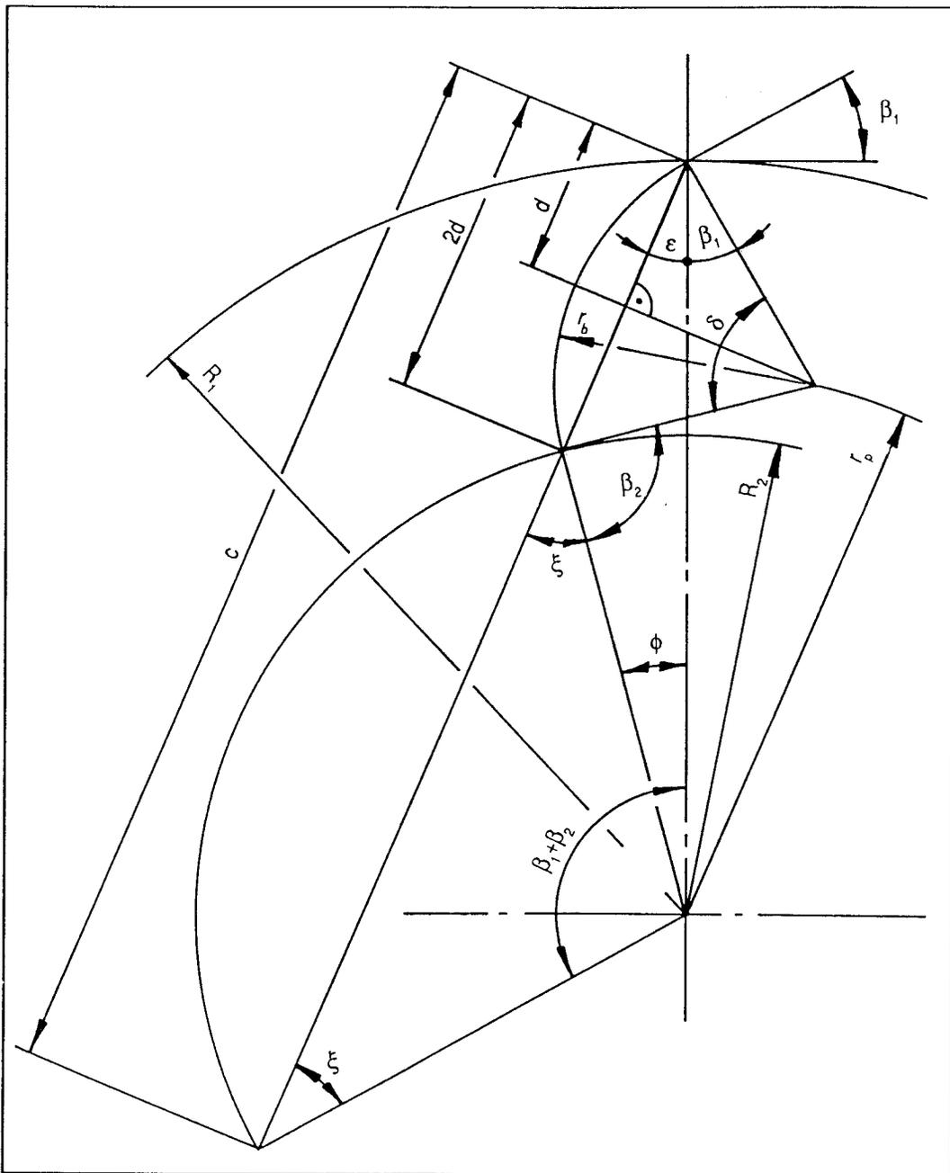
Fig. 1.9 : Construction of blade geometry
