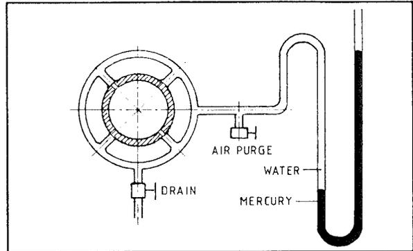
Fig. 3.8: Static pressure measurement in a pipe
