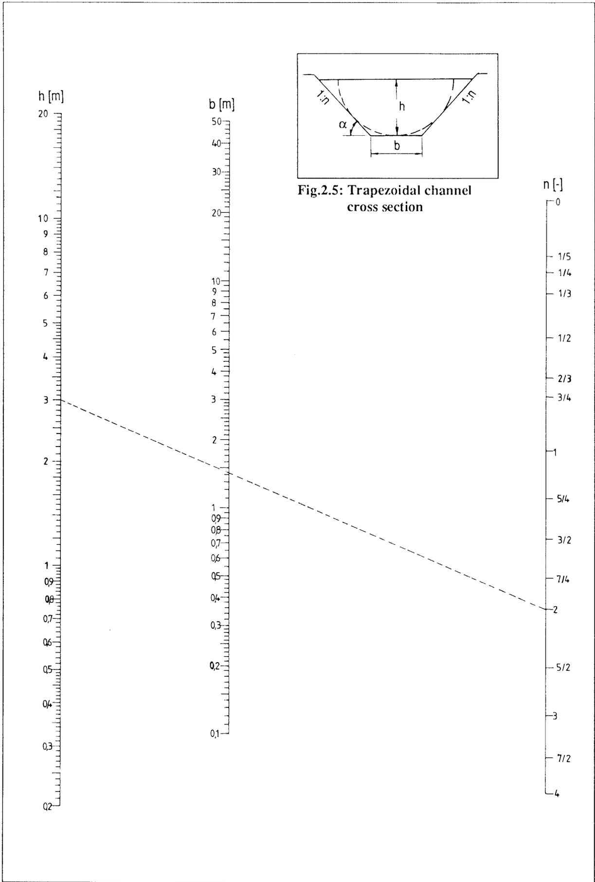
Fig. 2.4: Nomogram for optimal channel sections
