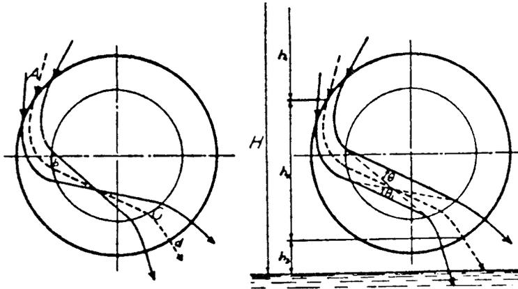
Figure 3. Interference of filaments of flow through wheel
