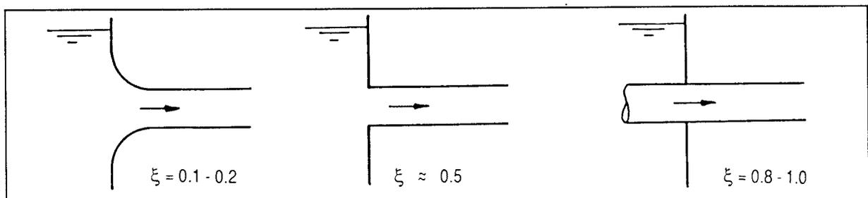
Fig. 2.11: Entrance loss resistance coefficients
