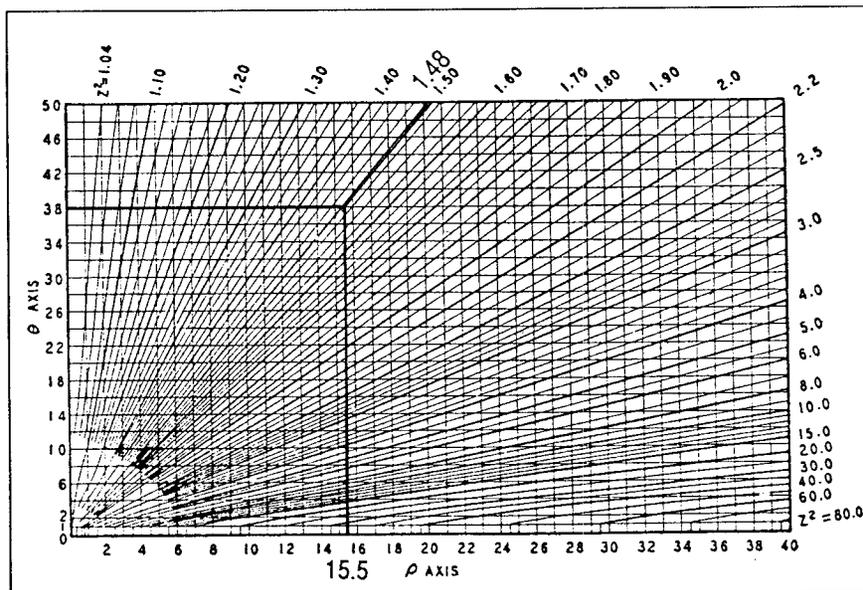
Fig.: 2.17: ALLIEVI chart: pressure rise for uniform gate closure and simple conduits ( large  $\rho$  and  $\theta$  )
