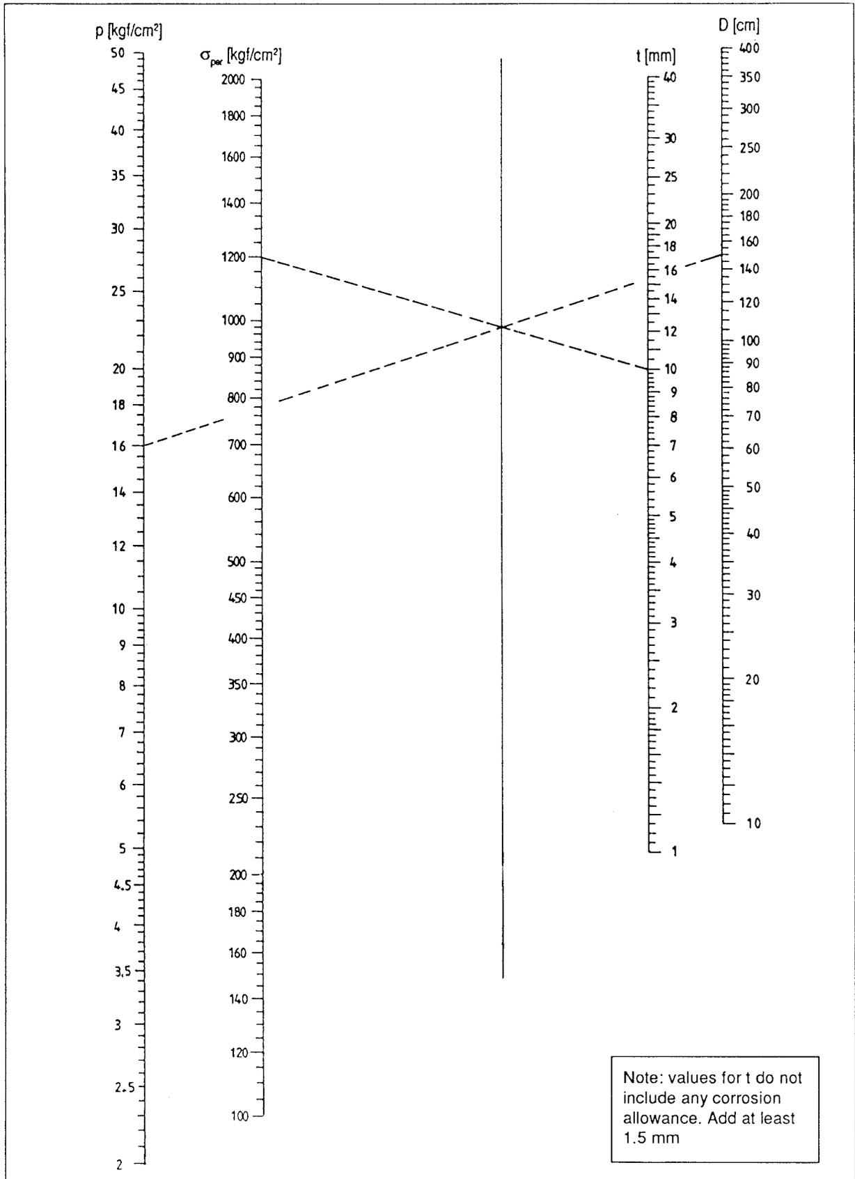
Fig.: 2.16: Nomogram for minimal penstock thickness
