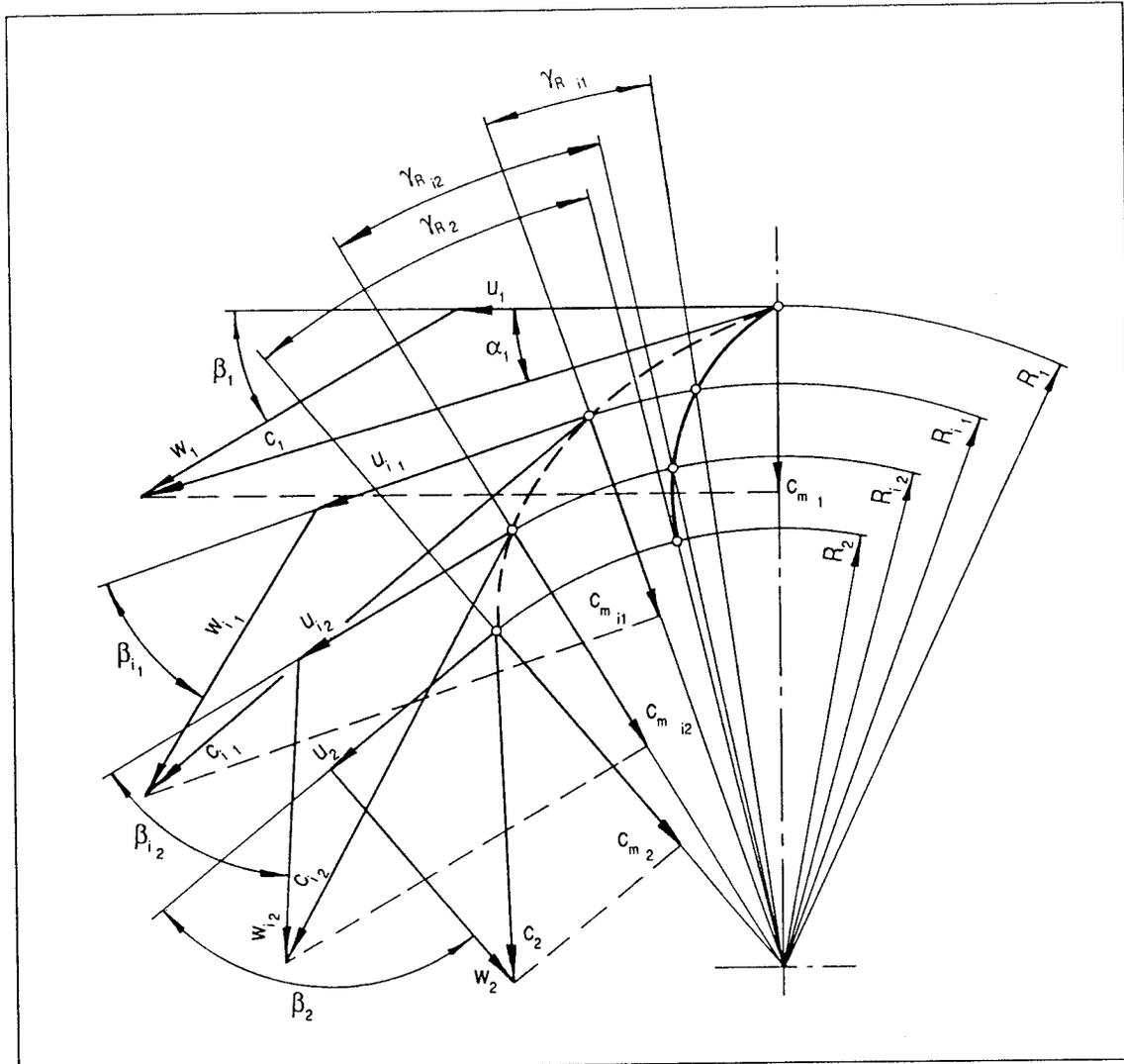
Fig. 1.7: Design of the absolute flow path in the first stage of a Cross Flow runner
