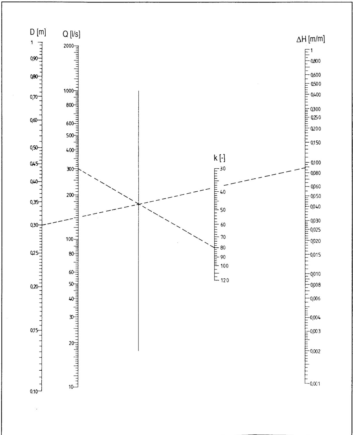
Fig. 2.9 : Nomogram for head losses in penstock
