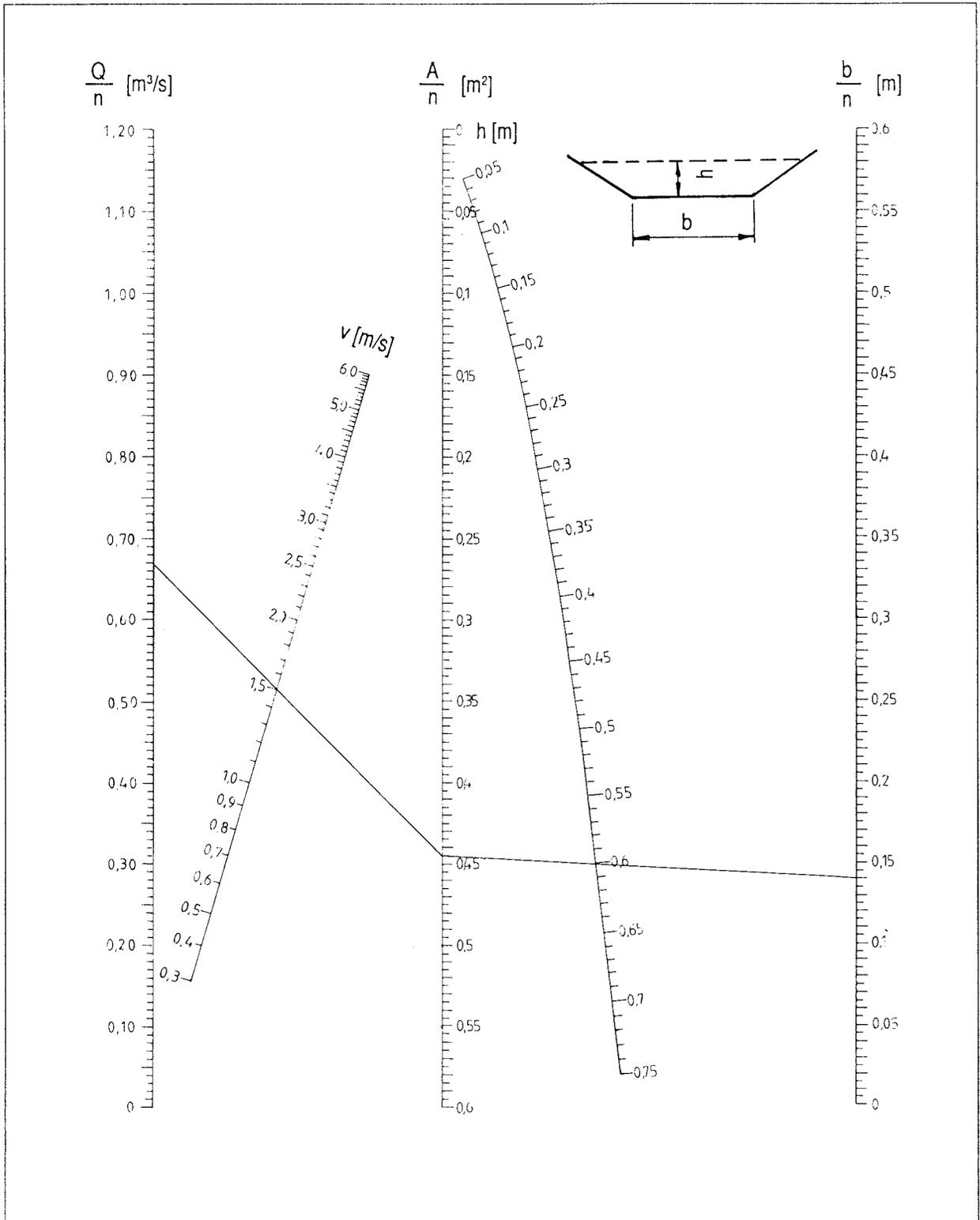
Fig. 2.6: Nomogram for trapezoidal channel cross sections
