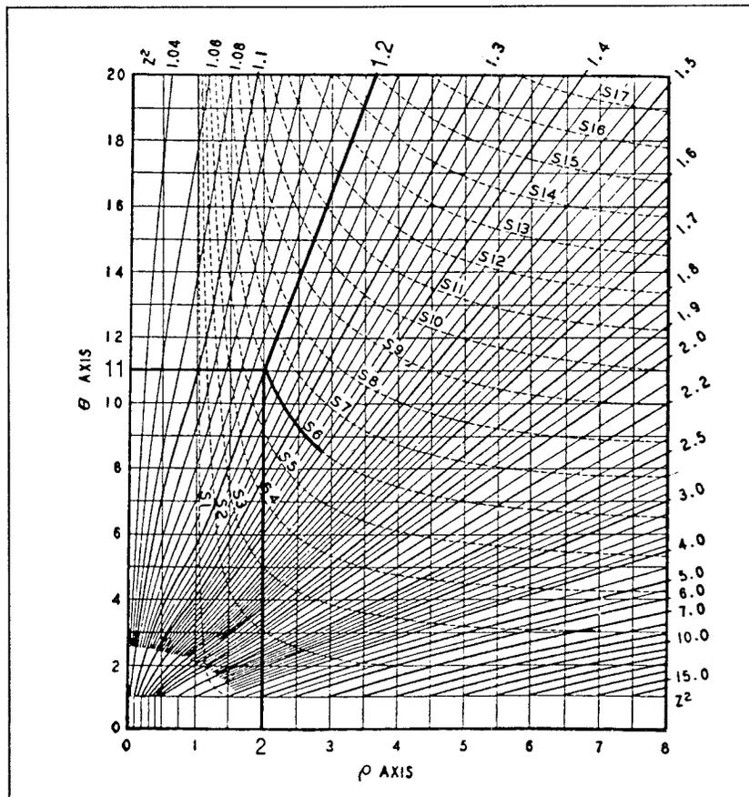
Fig. 2.19: ALLIEVI chart: pressure rise (medium  $\rho$  and  $\theta$ ) and wave cycle curves
