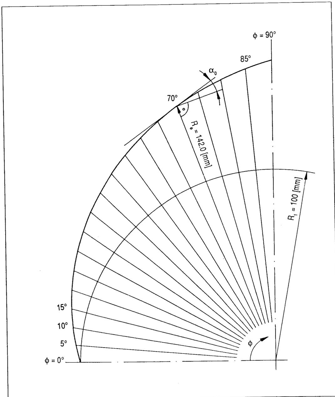
Fig. 1.13: Design of the logarithmical inlet spiral
