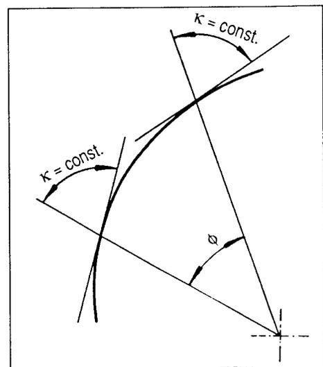
Fig. 1.12: Constant angle of the ideal inlet curve
