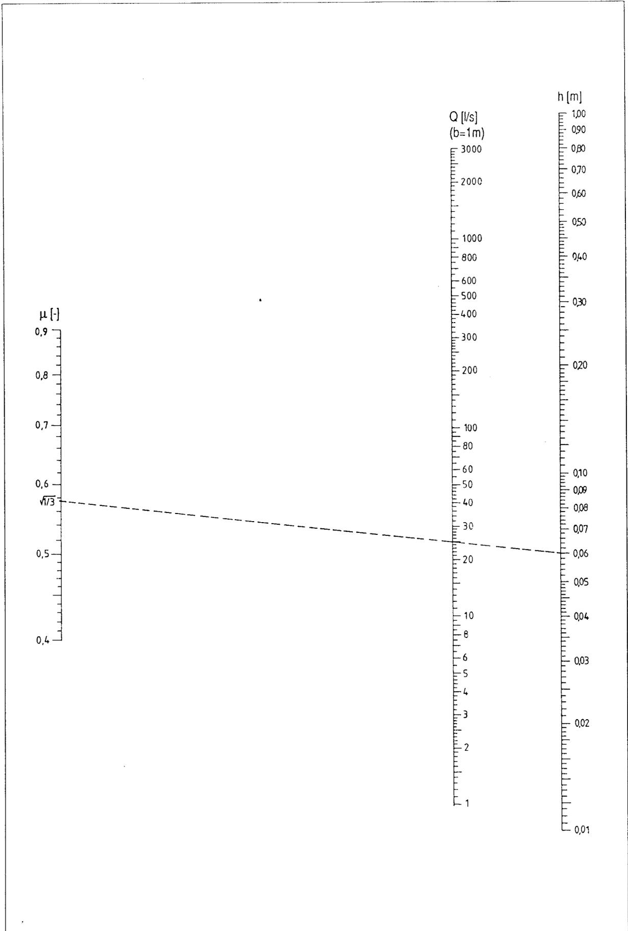
Fig.2.8: Nomogram for discharge measurement with weirs
