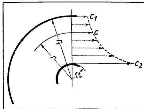
Fig. 1.3: Velocity distribution according to the law of angular momentum
