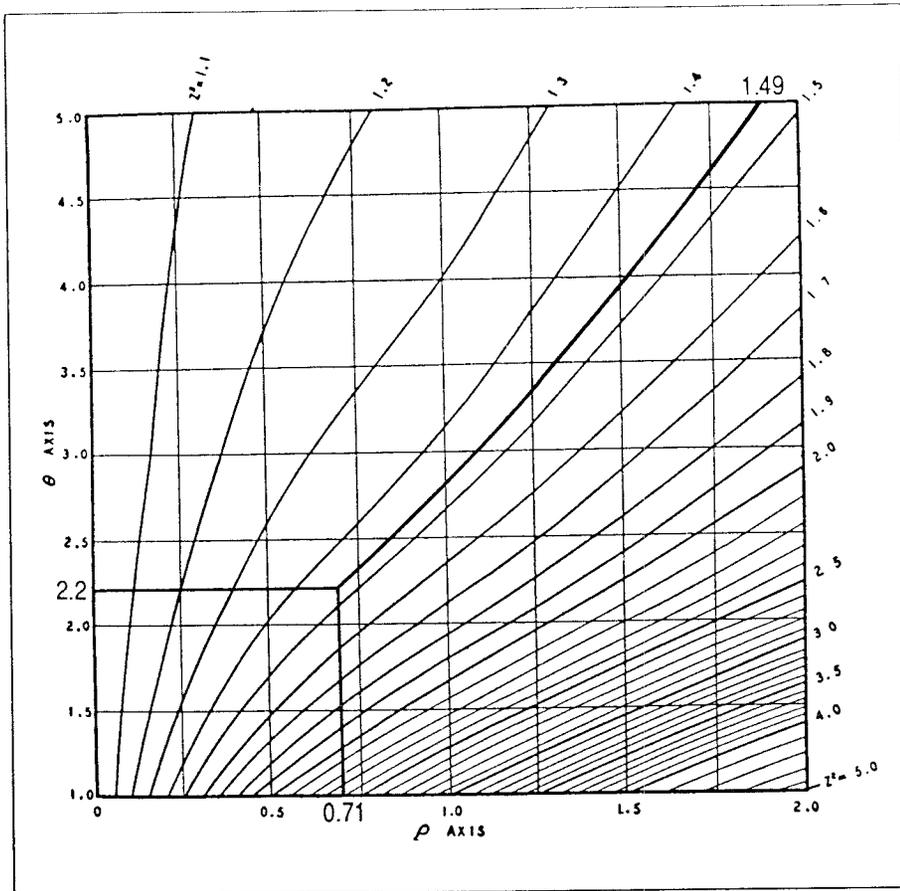
Fig. 2.18 :ALLIEVI chart: pressure rise for uniform gate closure and simple conduits ( small  $\rho$  and  $\theta$  )
