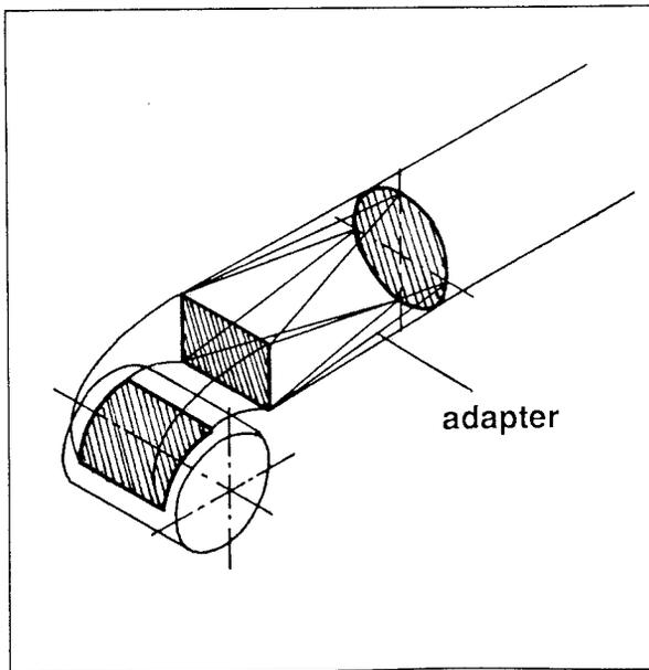
Fig. 1.10: Cross-sections of flow at the inlet of Cross Flow turbines
