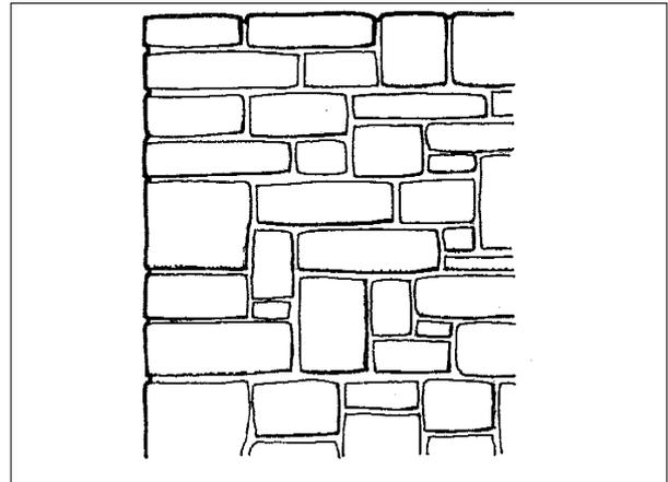
The rules for plumbing and lining are the same as for brick laying. It is advisable to hang one line for the inner wall and to work with two masons at the same time. One mason builds on the outside, the other on the inside of the line.
