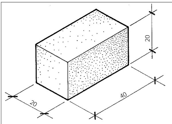
Horizontal and vertical joints are increased to 15mm because of the reasons mentioned above (levelling, placing the blocks completely in mortar, and to avoid uneven or incomplete support). The increased size of cement blocks in comparison to bricks
