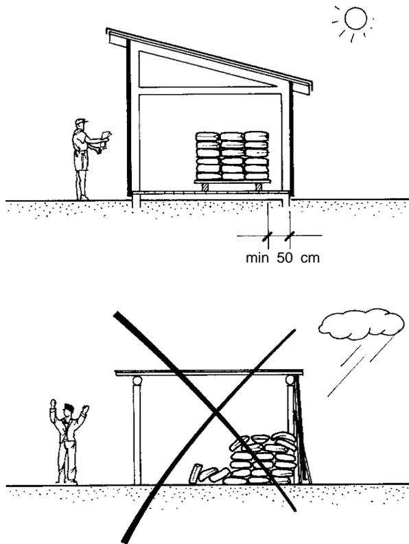
This is especially important in humid climates. The old stock should always be used before the new one. Cement can be expected to lose from its potential strength because of storage time as follows:
