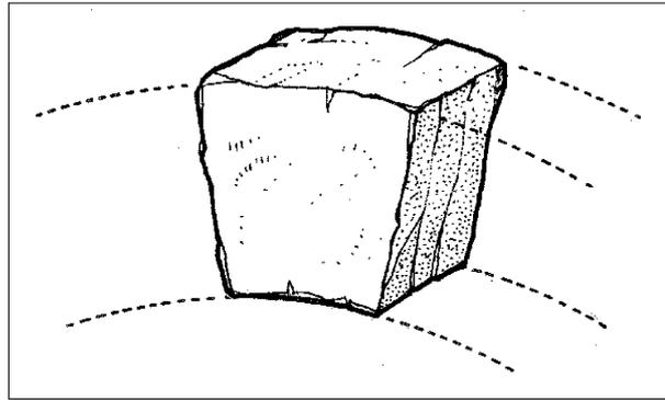
Unlike the cornerstone the arch stone is shaped like a wedge and is more difficult to shape than any other stone, because it has to be shaped to specific measurements.
