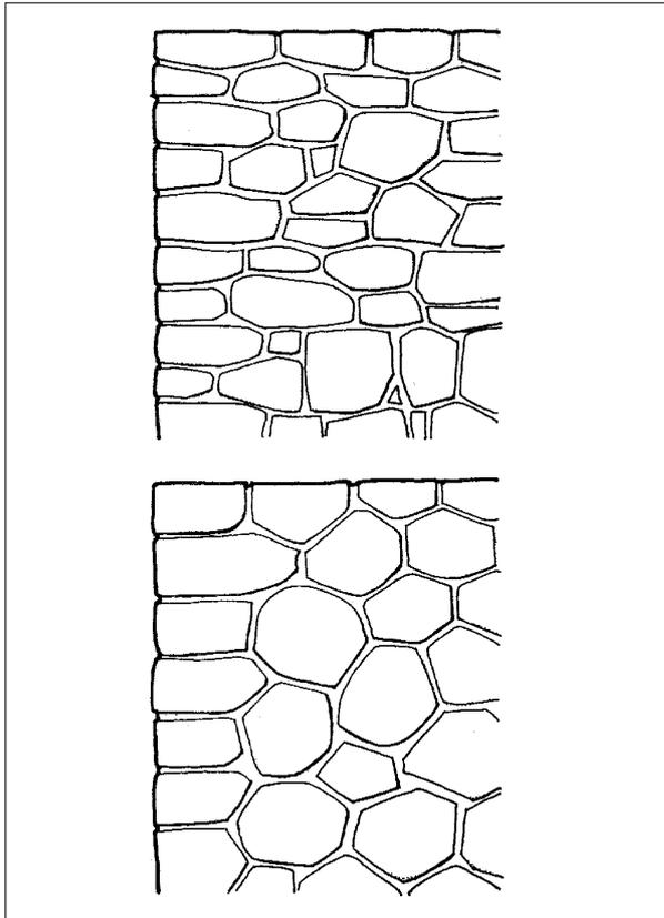
Uncoursed rubble masonry needs relatively little shaping and less precise jointing work. The layout and building of the structure will show clearly the builder's skill. Therefore, it is important to train builders in the special subject of stone masonry work. This kind of stone masonry uses all sizes of stones whose faces, joints and beds are roughly shaped. No attention is given to maintain level courses.
