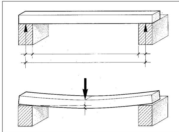
By embedding steel bars in the concrete, advantage is taken of these properties to improve the load carrying capacity of the structure. The steel is placed in the concrete that is subjected to tension but also to avoid cracks due to shrinking.
