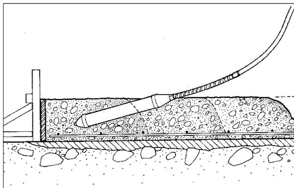
ment, to avoid vibration on the formwork or reinforcement. The vibration can cause holes and therefore weaken the structure.
