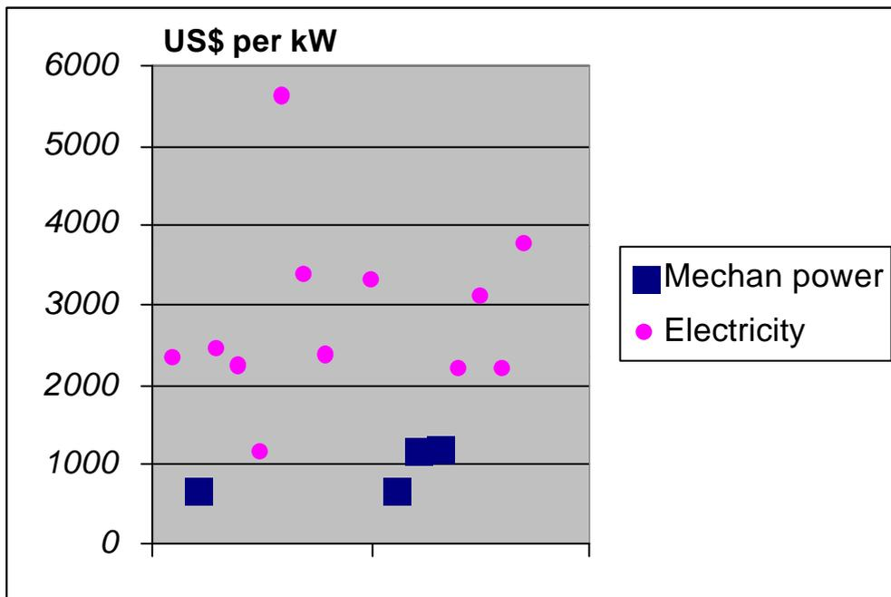
Electricity generation schemes, as expected have a higher installed cost per kW. there are also some differences between countries and even within the same country which might be explained by the following parameters:
