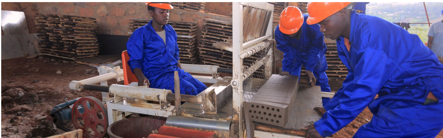
Semi-mechanised brickyards offer improved working conditions, protected from smoke, dust and excessive heat exposure. Work can be executed by women and men equally. The industrial machines recommended by the project can produce up to 10,000 green bricks per day.
