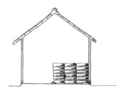
Wrong: Storing directly on the floor and on the outer wall
