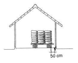
Good Storing on timber pallets and no contact with outer walls
