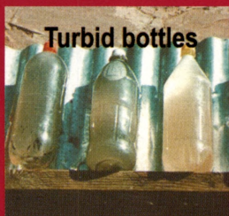
Bottles with low UV-transmittance: old, scratched, blind and coloured bottles.
