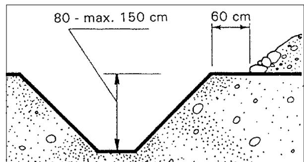
loose ground correct excavation
