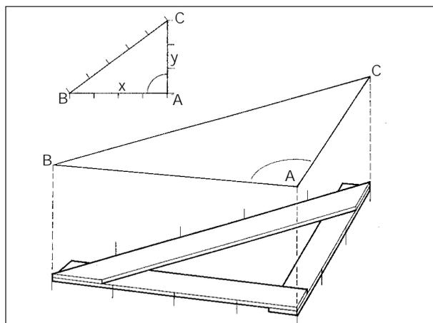
right angle is found at point A formed by the lines x and y.
