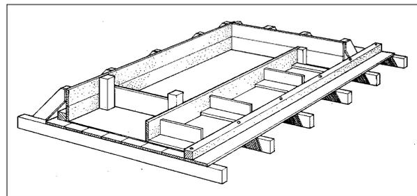
All form work material (planks, boards, steel etc.) and element form work (moulds) are sprinkled with water before placing concrete. After striking or dismantling, the form work is cleaned and eventually oiled as well as properly stored and protected from sun and rain. This will guarantee the use of many times.
