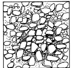
If possible use coarse grained sand and never the fine sieved sand used for masonry work. Reminders of coarse sand from sieved masonry sand can be added to the aggregates when mixed with coarse grained sand.
