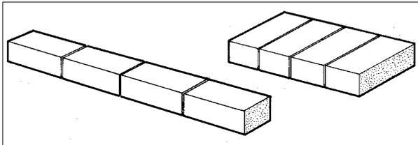
Bricks can be laid in a variety of bondings. To prevent the crushing of bricks use bondings of as many full bricks as possible, three quarter and half bricks. There are other bondings possible, but they are not used for water supply structures.
