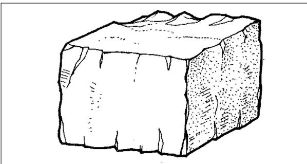
The two faces should be squared and shaped with chisel and club hammer to a plain surface, or at least hammer dressed to make accurate plumbing possible.
