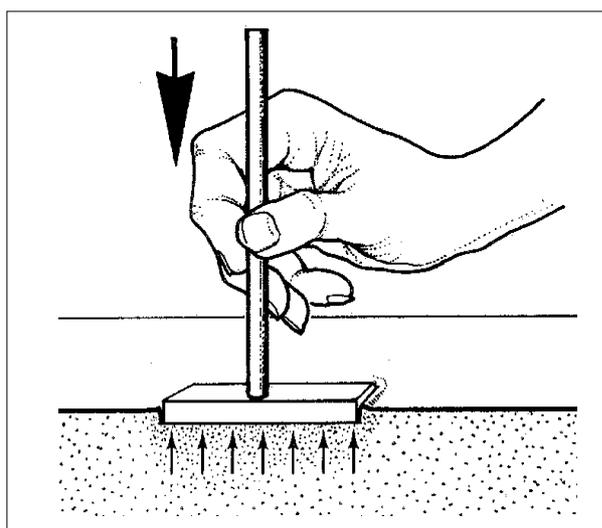
According to the weight of the structure and the type of the soil the size of the foundation needs to be designed. At too small foundation cannot be used in a low capacity bearing soil, it will sink into the soil.
