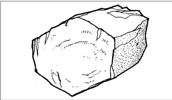
Stones built between corner stones are called line stones. They should be (but not necessarily) plain surfaced. The combination of plain surface corners and rough hammer dressed line stones give the stone masonry an attractive appearance.
