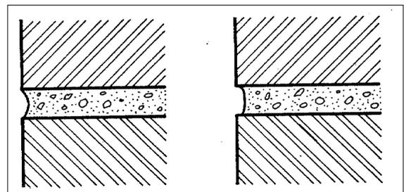
Made with pointing tool or a piece of small pipe. Two centimeters of the set mortar is scratched out of the joints and later filled with pointing mortar of a ratio 1:3 to 1:2 as shown in the drawing. This pointing is work intensive and expensive, but has a big influence on the quality of the structure.
