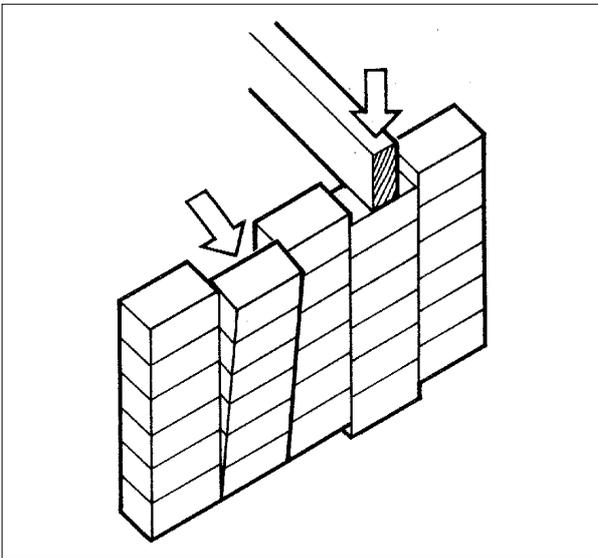
Bonded walls provide stability and resistance to the side thrust, as seen in the figure above. The bond can be selected to give an attractive appearance to the wall face.
