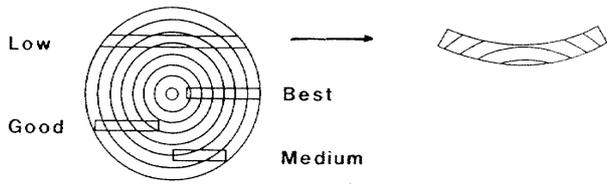
beams or boards. The part of the trunk from which they are cut and the slope of grain have great effect on the quality of the product. Therefore, when selecting timber, the direction of the grain has to be observed.
