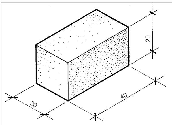
Horizontal and vertical joints are increased to 15mm because of the reasons mentioned above (levelling, placing the blocks completely in mortar, and to avoid uneven or incomplete support). The increased size of cement blocks in comparison to bricks
