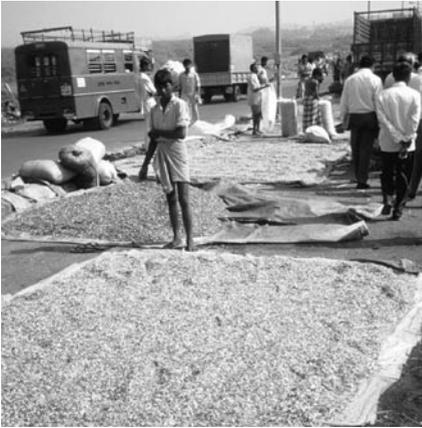
This recycled plastic is being dried after having been sorted according to colour, shredded and washed.
