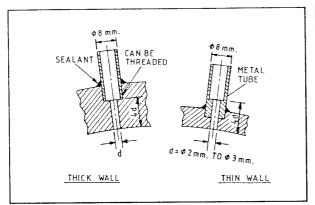
Fig. 3.9: Single pressure tapping in PVC pipe
