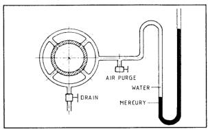
Fig. 3.8: Static pressure measurement in a pipe
