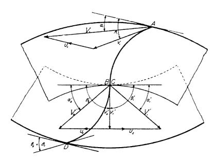
Figure 6. Composite velocity diagram
