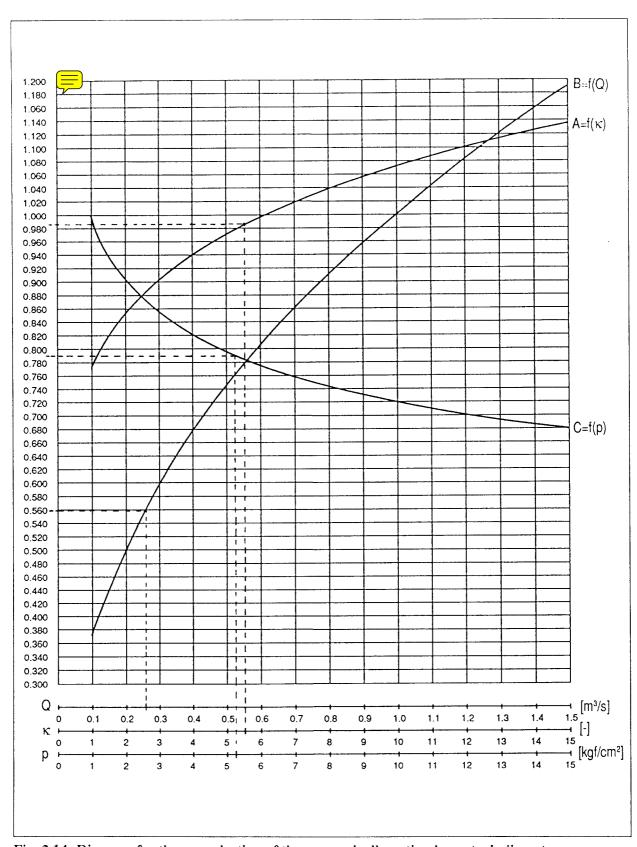
Fig. 2.14: Diagram for the pre-selection of the economically optimal penstock diameter
