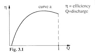
turbine characteristics of a properly sized machine for a maximum discharge of Q = 1.
