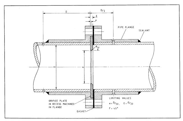
Fig 3.10: Orifice meter in PVC pipe
