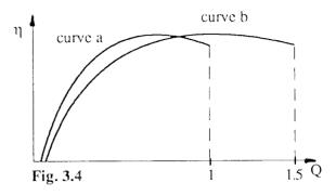
It is now evident, that curve b represents the turbine characteristics of a 50% oversized machine as compared to curve a. Which machine is the better choice only depends on the available discharge Q.
