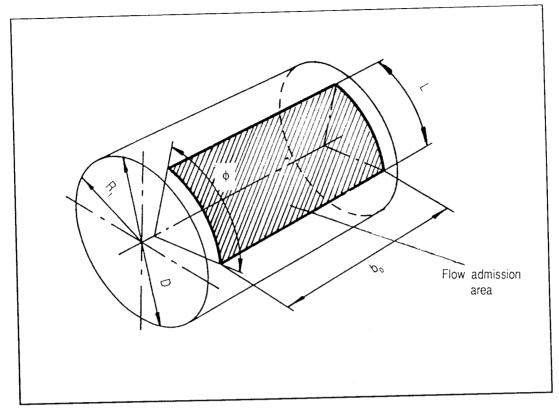
Fig. 1.14: Flow admission area of a Cross Flow turbine
