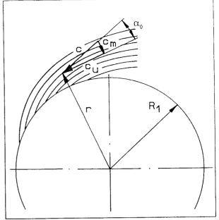
Fig. 1.11: Ideal flow conditions in the inlet
