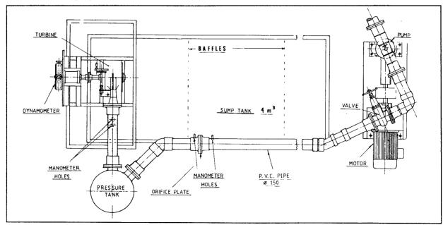
Fig. 3.7: Plan view of turbine test rig layout
