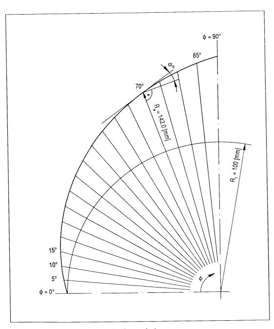
Fig. 1.13: Design of the logarithmical inlet spiral
