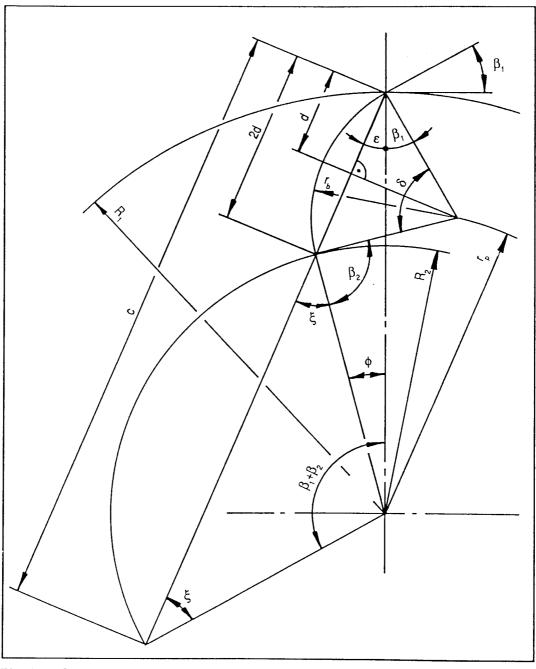
Fig. 1.9: Construction of blade geometry
