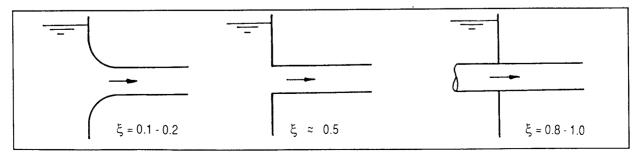
Fig. 2.11: Entrance loss resistance coefficients
