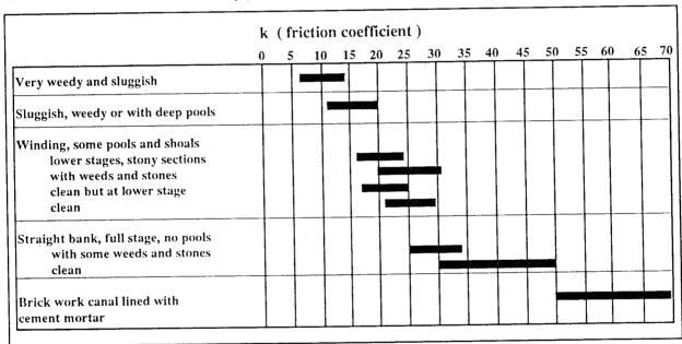
Fig. 2.1: Friction coefficients k of STRICKLER
