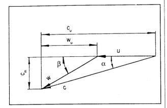
Fig. 1.5: Terms used in velocity triangles
