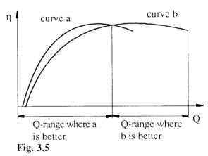
The following example shows dry season conditions where only a limited amount of water is available. In such a case, the efficiency drop of an oversized machine as compared to a properly sized one may be significant and may possibly mean a temporary shut down of the entire plant.
