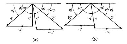
Figure 7. Velocity diagrams
