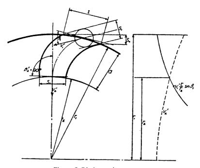
Figure 5. Blade spacing
