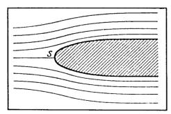
Fig. 1.2: Rounded leading edge of an object imerged in a flowing fluid. S = stagnation point
