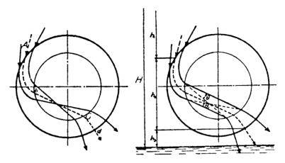
Figure 3. Interference of filaments of flow through wheel
