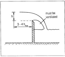
Fig. 2.7: Details & notations on rectangular weirs (Illustrations from WMO [10])
