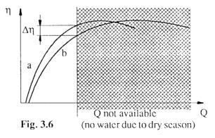
The explanations given also make it clear why turbine designers try hard to develop machines with a flat efficiency curve. The object being to achieve a high efficiency over a wide range of discharge.
