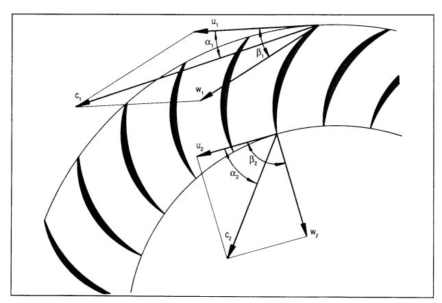
Fig. 1.4: Velocity triangles in a runner with peripheral blades
