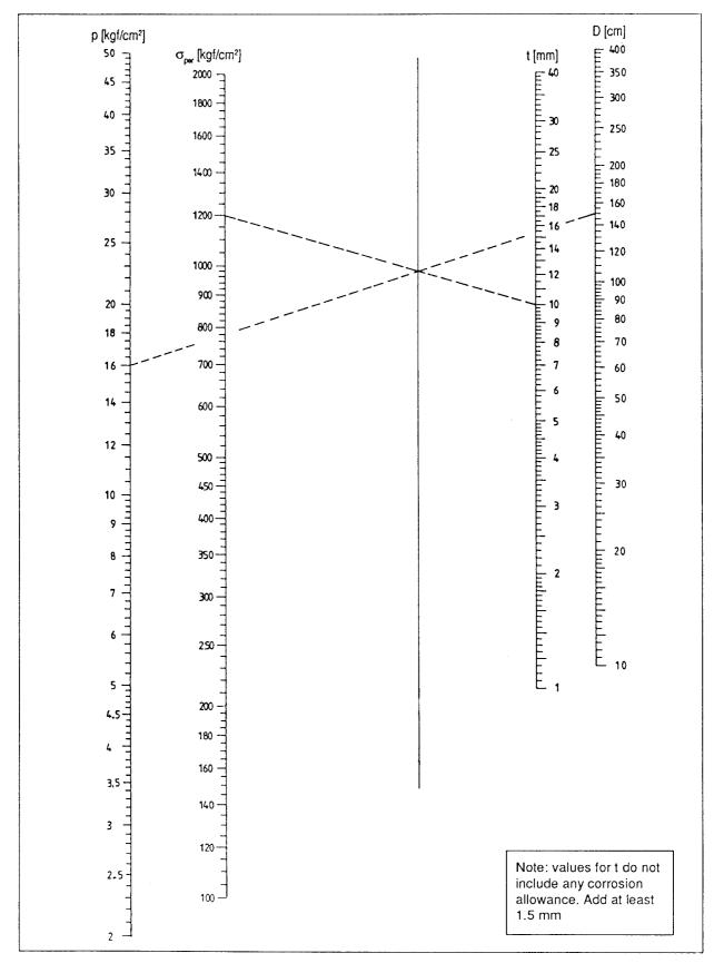
Fig.: 2.16: Nomogram for minimal penstock thickness
