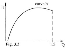
turbine characteristics of a properly sized machine for a maximum discharge of Q = 1.5.
