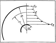
Fig. 1.3: Velocity distribution according to the law of angular momentum
