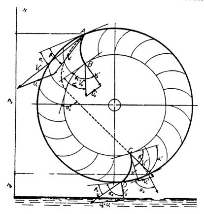
Figure 2. Path of water through turbine
