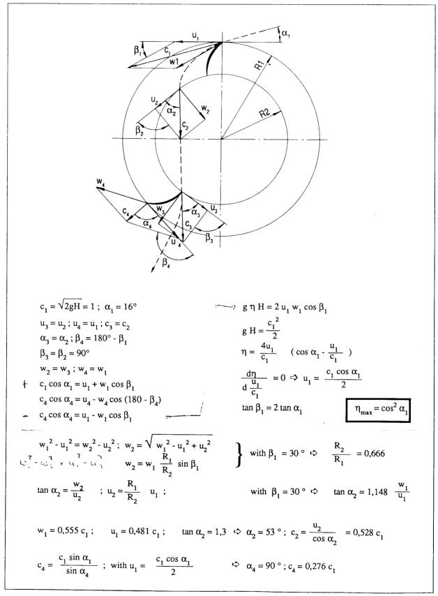
Fig. 1.6: Velocity triangles and related formulae for a Cross Flow turbine
