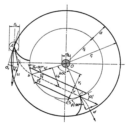
Figure 8. Path of jet inside wheel
