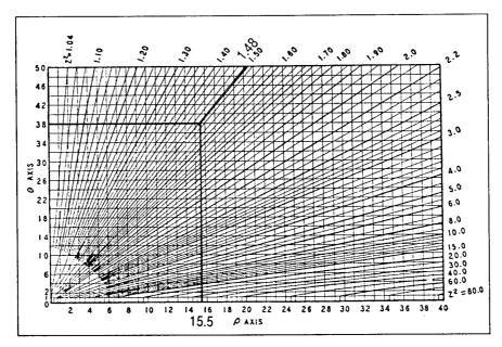
Fig.: 2.17:ALLIEVI chart: pressure rise for uniform gate closure and simple conduits ( large  $\rho$  and  $\theta$  )
