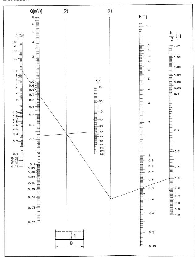
Fig. 2.3: Flow in rectangular canal cross sections
