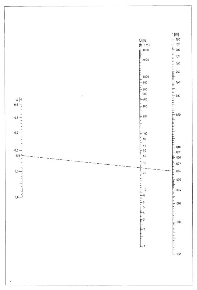
Fig.2.8: Nomogram for discharge measurement with weirs
