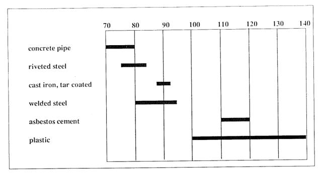
Fig. 2.10: Friction coefficients k for penstock materials according to STRICKLER (note that higher k-numbers mean lower losses)
