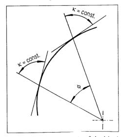
Fig. 1.12: Constant angle of the ideal inlet curve
