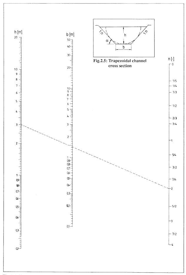
Fig. 2.4: Nomogram for optimal channel sections
